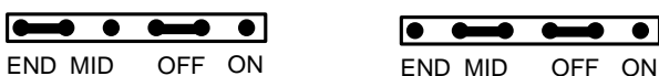
Diagrams showing CDR-IF jumper settings for : a) termination OFF (MID), b) termination ON (END). Note Jumper J1 not shown.
